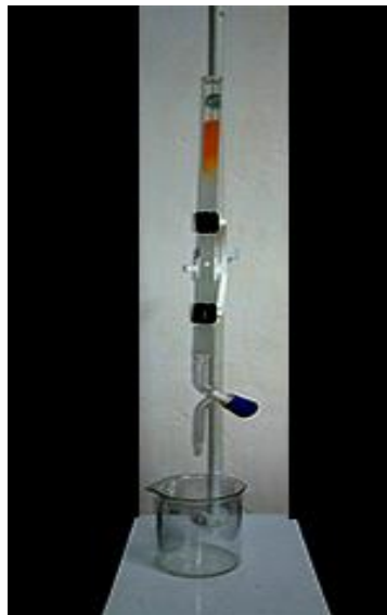
Figure 30. Silica gel (60-120 mesh) column loaded with the crude pigment extract. Purified fraction was eluted with 5 % ethyl acetate in n -hexane.
