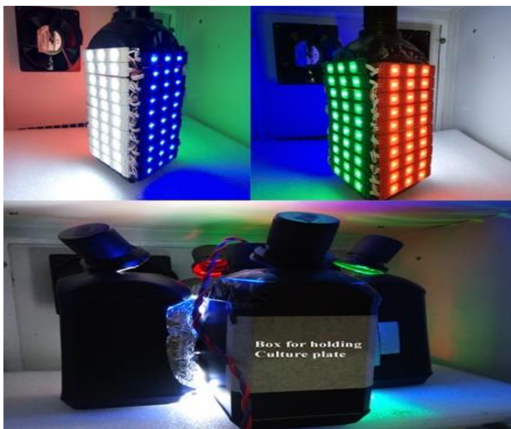
Figure 9. Box type-black chamber setup for providing different LED light conditions
