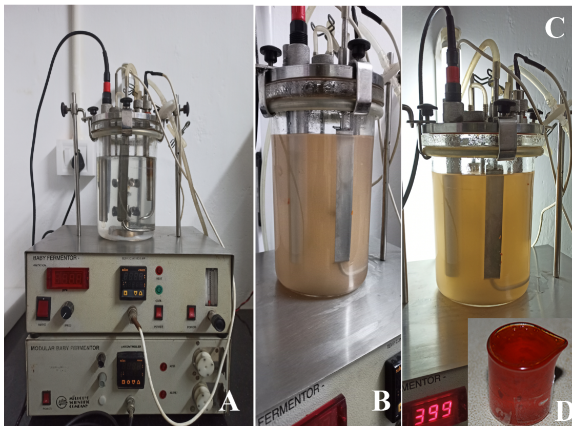
Figure 29. Bioreactor setup for the large scale production of prodigiosin having DEHP as the only carbon source for A. denitrificans SP1. A) Bioreactor setup before inoculation. B) & C) After 8 days of incubation at RSM optimized cultural conditions. D) Extracted prodigiosin.
