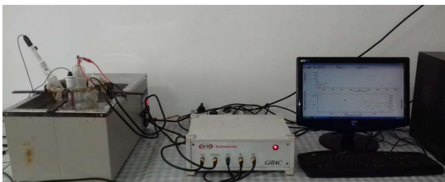
Fig2.5 experimental set up for electrochemical measurements
