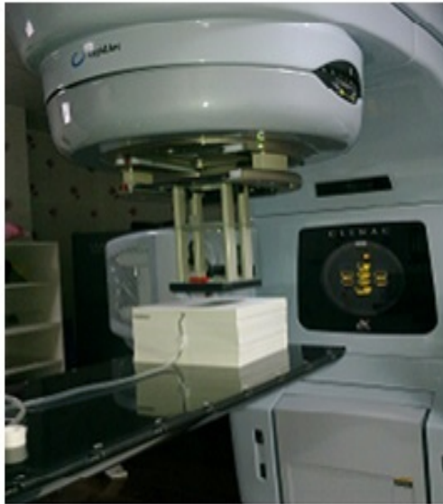
Figure 6.3: Experimental setup using plastic water phantom in LINAC.
