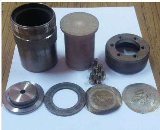
Fig. 2.2: Parts of a typical autoclave used for hydrothermal process.
