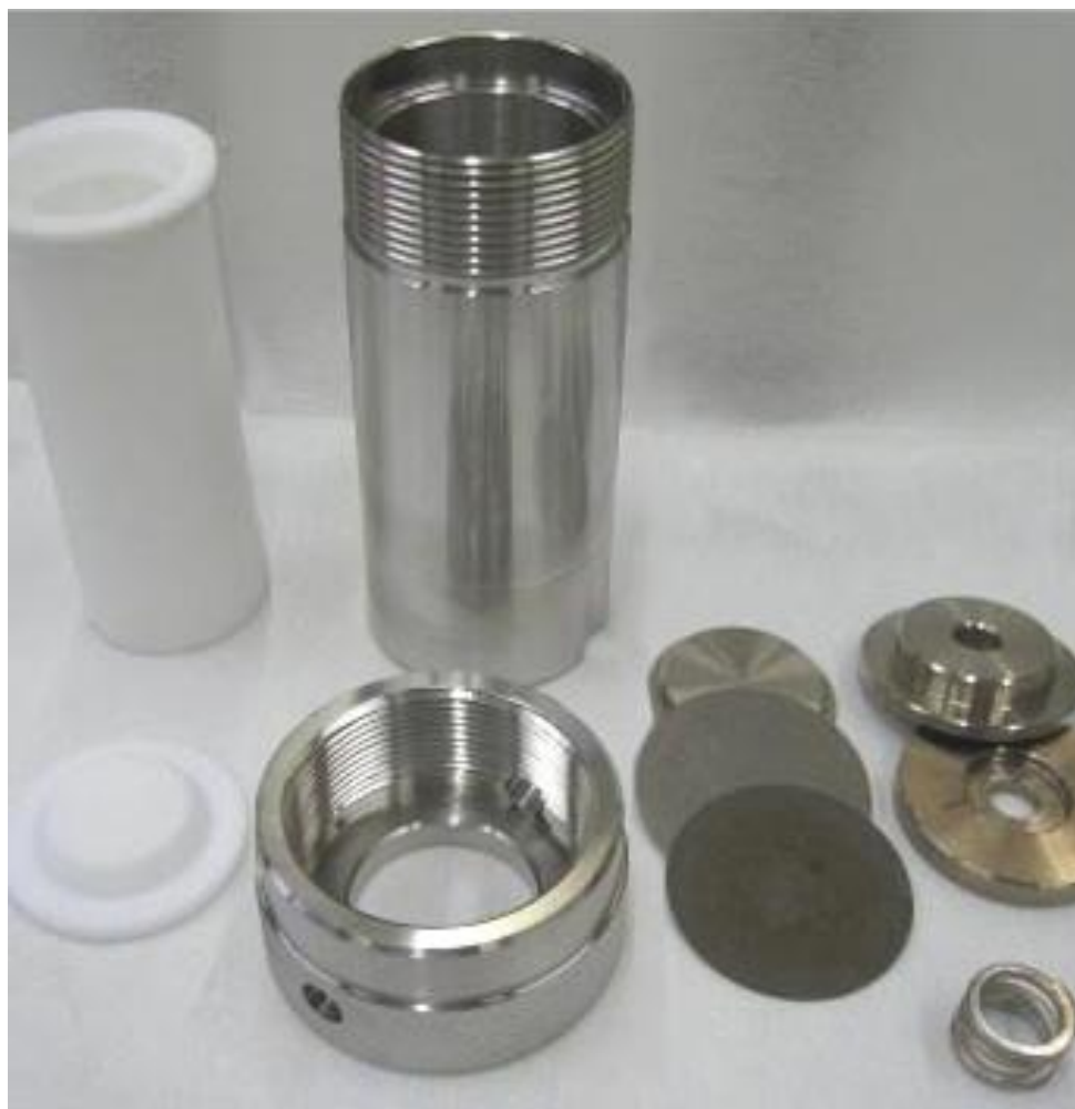
Figure 2.1 Hydrothermal setup for the synthesis of titania nanostructures
