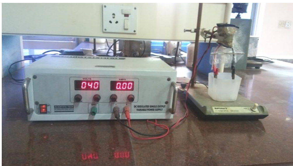
Figure 2.2 Anodization setup for the synthesis of titania nanotubes
