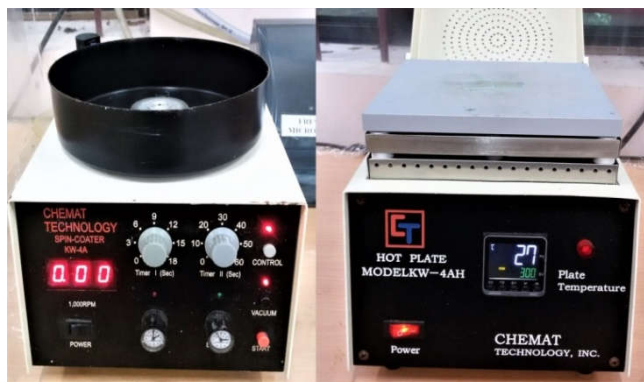
Fig. 2.6 Spin coater (Chemat KW4) used for the present study along with hot plate
