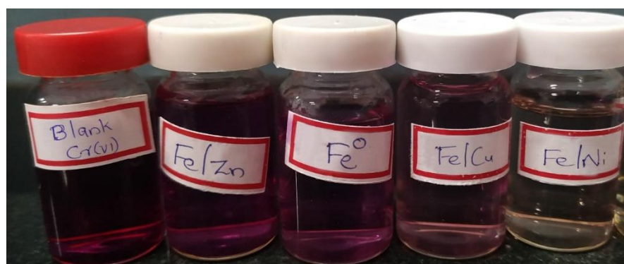
Figure 3.7 Photographs of \text{Cr(VI)} removal using \text{Fe}^0 , \text{Fe/Ni} , \text{Fe/Cu} and \text{Fe/Zn} nanoparticles
