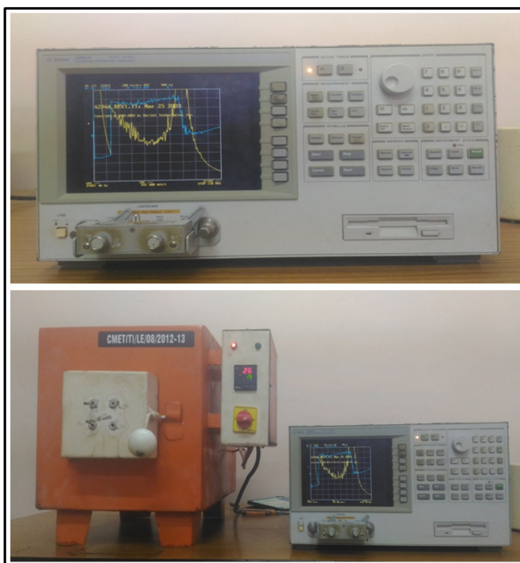
Figure 2.12 Set-up for dielectric characterisation
