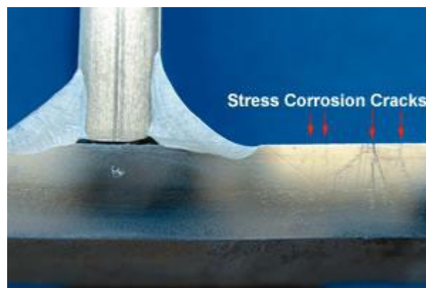
Fig. 1.5: Stress-corrosion cracking of mild steel
