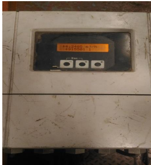
Fig 3.7 Digital Flow meter used in the study
