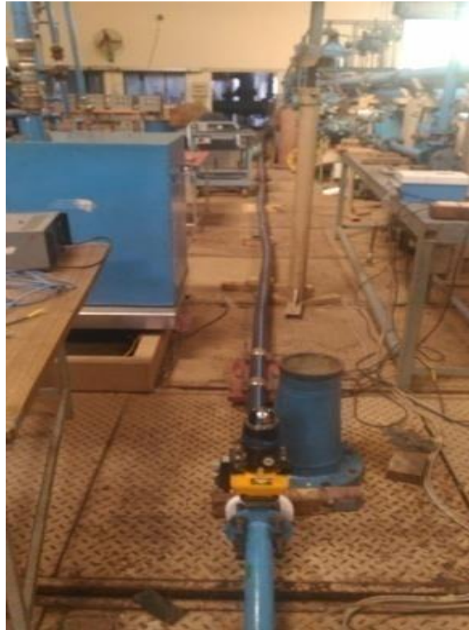
Fig. 3.16 Experimental installation for conducting experiments in HDPE Pipe
