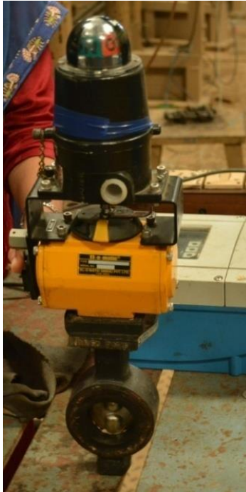
Fig. 3.9 Pressure actuated Quick Acting Valve (QAV)
