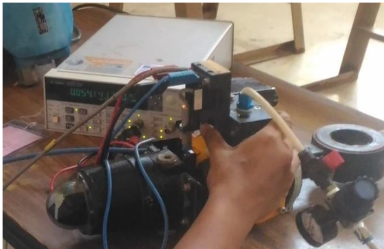
Fig. 3.10 Arrangement for the determination of closure time of Quick Acting Valve
