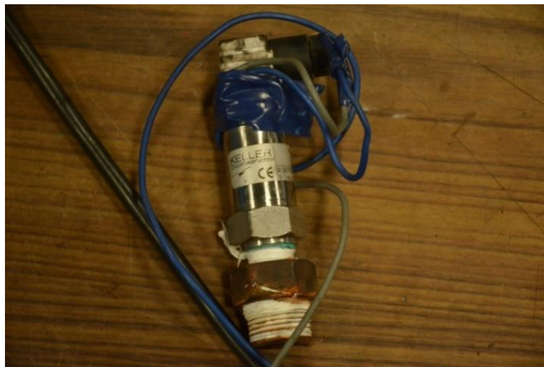
Fig. 3.6- Pressure Transducer Range 0-30 bars
