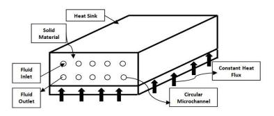
Fig 1.4 Example for Double Layer Microchannel (CF)
