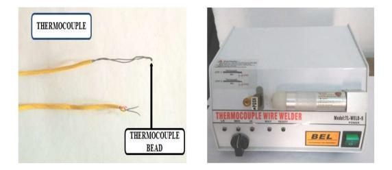
Fig 3.19 Thermocouple
