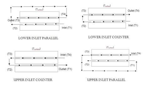
Fig 3.36 Schematic of Different Series Flow Configurations (EXPERIMENT)
