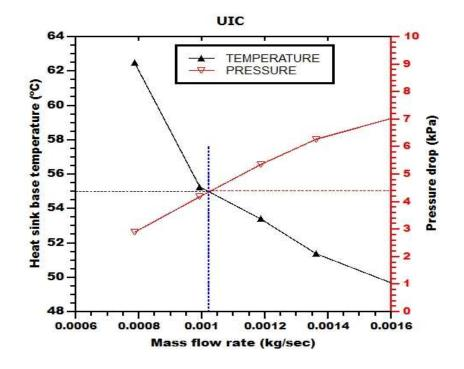
Fig 4.52 Variation of Heat Sink Base Temperature and Pressure Drop with the Mass Flow Rate (UIC)
