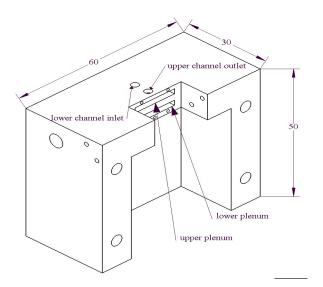
Fig 3.16 Schematic of the Teflon covers
