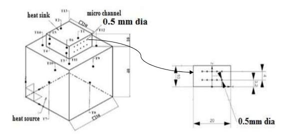
Fig 3.26 Geometry of Test Section with Thermocouple Positions
