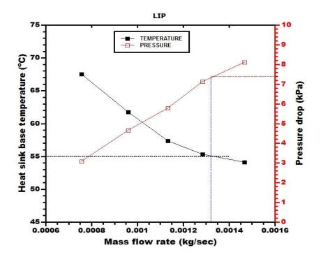
Fig 4.49 Variation of Heat Sink Base Temperature and Pressure Drop with the Mass Flow Rate (LIP)
