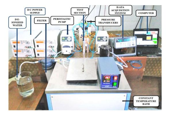
Fig 3.6 Photograph of Typical Experiment Setup
