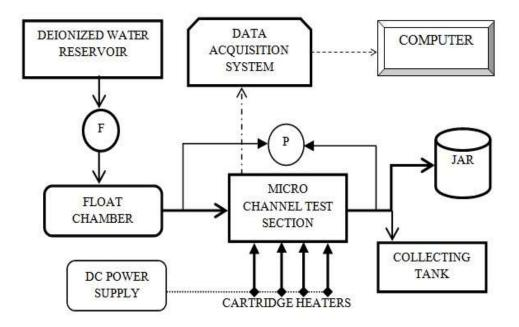
Fig 3.31 Schematic Flow Loop (GRAVITY FEED SYSTEM)
