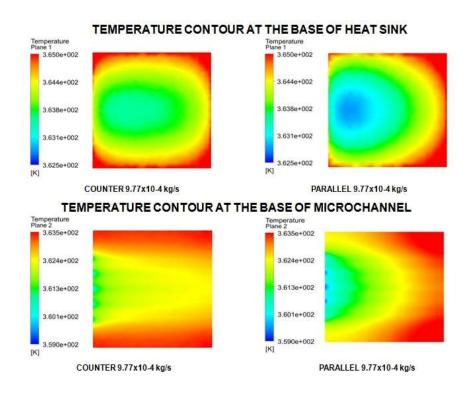
Fig 4.27 Temperature Contour (Case 1)
