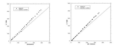
Fig A 2 – 3, Digital manometer calibration curves
