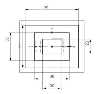
Fig 3.4 Schematic of the Computational Model used for Numerical Analysis
