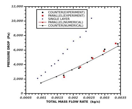
Fig 4.19 Total Pressure Drop with the Total Mass Flow Rate
