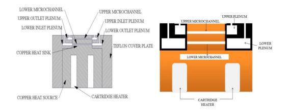
Fig 3.13 Sectional view of the Test Piece with Teflon covers.
