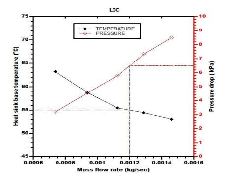
Fig 4.50 Variation of Heat Sink Base Temperature and Pressure Drop with the Mass Flow Rate (LIC)
