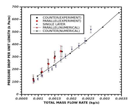
Fig 4.20 Pressure Drop per Unit Length with the Total Mass Flow Rate
