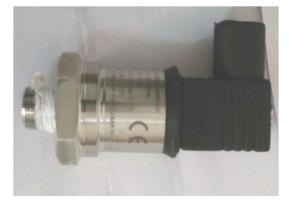
Fig 3.24 Pressure Transducer
