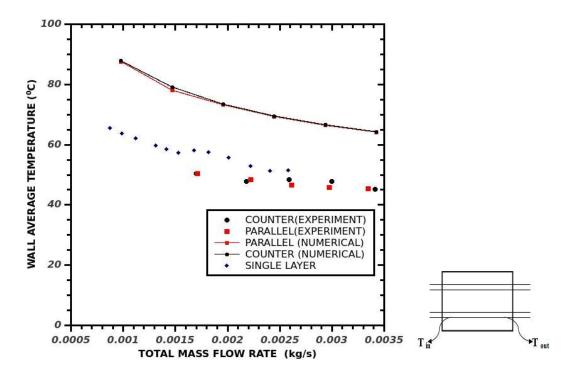
Fig 4.25 Wall Average Temperature with the Total Mass Flow Rate
