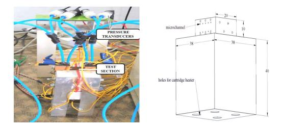
Fig 3.7 (a) Test section and Pressure Transducers
