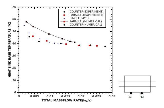
Fig 4.10 Heat Sink Base Temperature Vs the Total Mass Flow Rate
