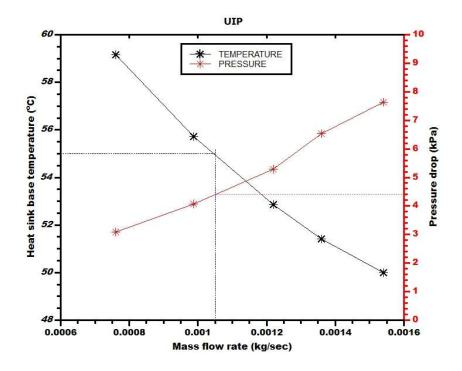
Fig 4.51 Variation of Heat Sink Base Temperature and Pressure Drop with the Mass Flow Rate (UIP)
