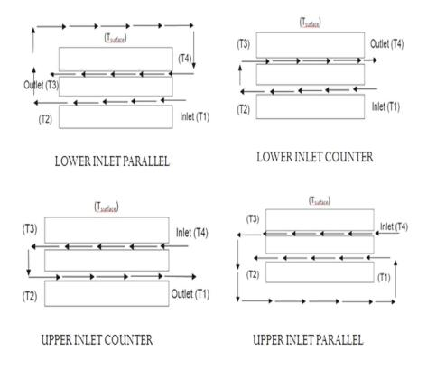
Fig 4.39 Schematic of Different Series Flow Configurations (EXPERIMENT)
