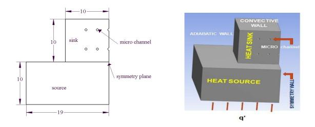
Fig 3.2 (a) Schematic of the Test Section. Fig 3.2 (b) Computational Domain for Numerical Analysis
