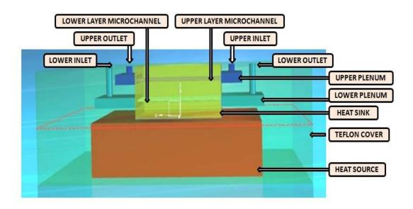
Fig 3.3 Computational Model used for Numerical Analysis
