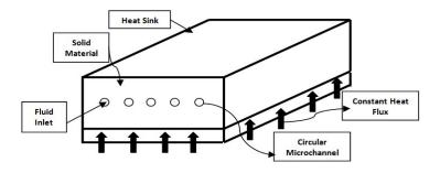
Fig 1.3 Example for Single Layer Microchannel
