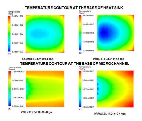
Fig 4.32 Temperature Contour (Case 6)
