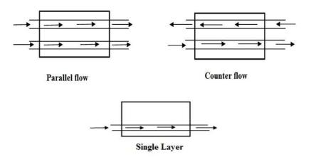
Fig 4.3 Flow Configuration for Experiment Study
