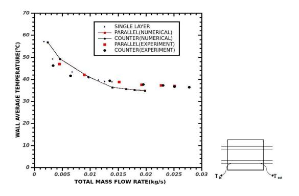
Fig 4.9 Wall Average Temperature Vs the Total Mass Flow Rate
