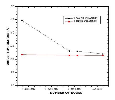
Fig 4.34 Outlet Temperature Vs Number of Nodes
