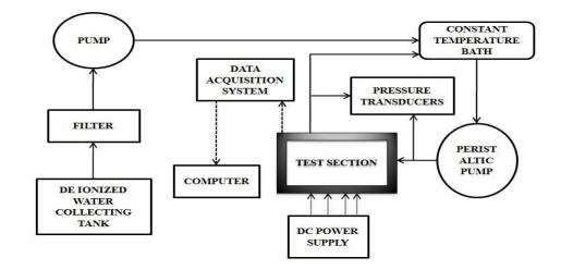
The schematic flow loop of the actual experiment setup is shown in Fig.3.5.
