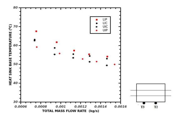
Fig 4.47 Heat Sink Base Temperature with the Total Mass Flow Rate
