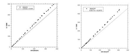
Fig A 2 – 2, Digital manometer calibration curves
