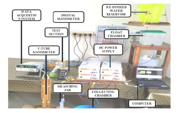
Fig 3.32 Pictorial View of Experiment Setup
