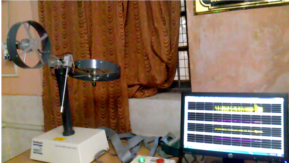
Figure 5.12: Real time setup for 2-dof TRMS using non-linear SMC with super-twisting control and non-linear sliding surface design
