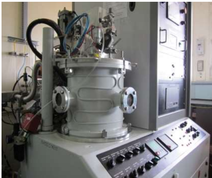
Figure.2.5 Photograph of the Two target Sputtering System
