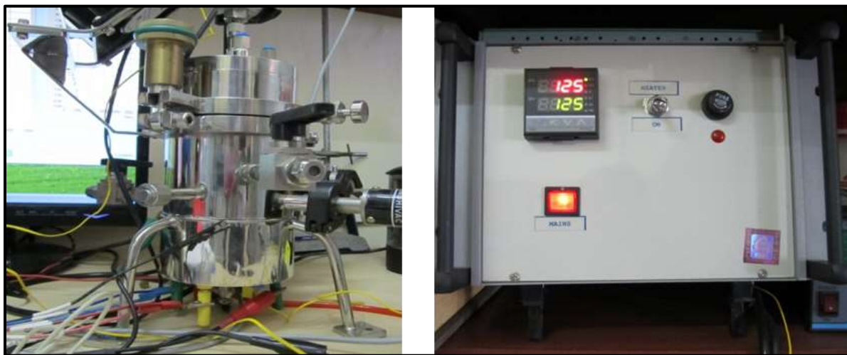
Figure.6.3 Photograph of (a) gas sensing chamber and (b) PID controller
