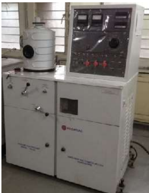
Figure 2.8 Photograph of the thermal evaporation system
