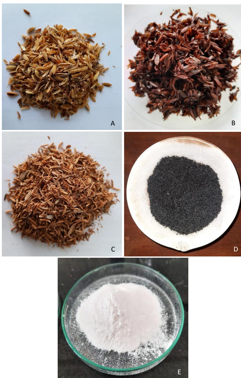
Figure 3.2.5. Showing (A) Untreated rice husk, (B) Acid leached and washed rice husk, (C) Dried acid pretreated rice husk, (D) Incomplete combustion of rice husk samples at incineration temperature below 200 °C showing presence of carbon and (E) Rice husk-derived silica obtained after controlled incineration
