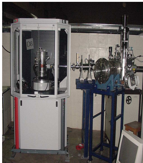
Fig. 2.4. X-ray diffractometer machine used for this work.
