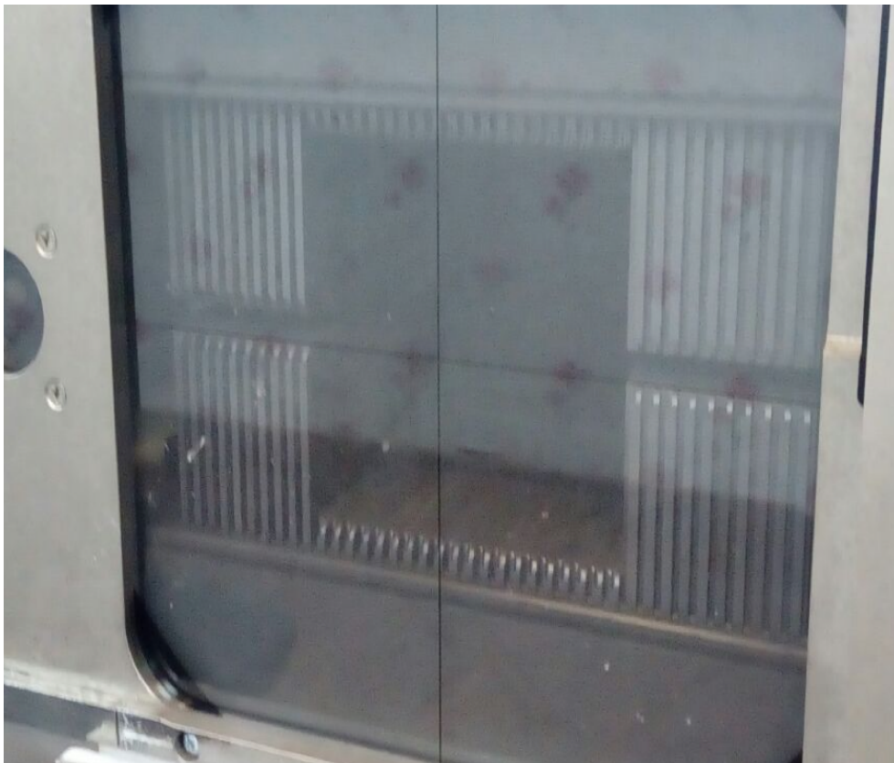
Figure 1.6: Diagram of a Multileaf collimators attached to Clinac iX
