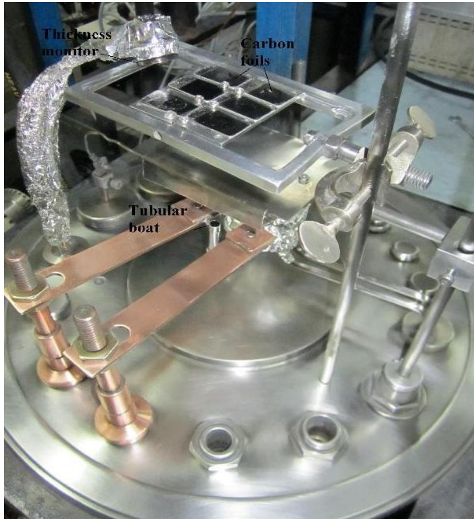
Figure 3.3: Set-up for Tl deposition on carbon foils.
