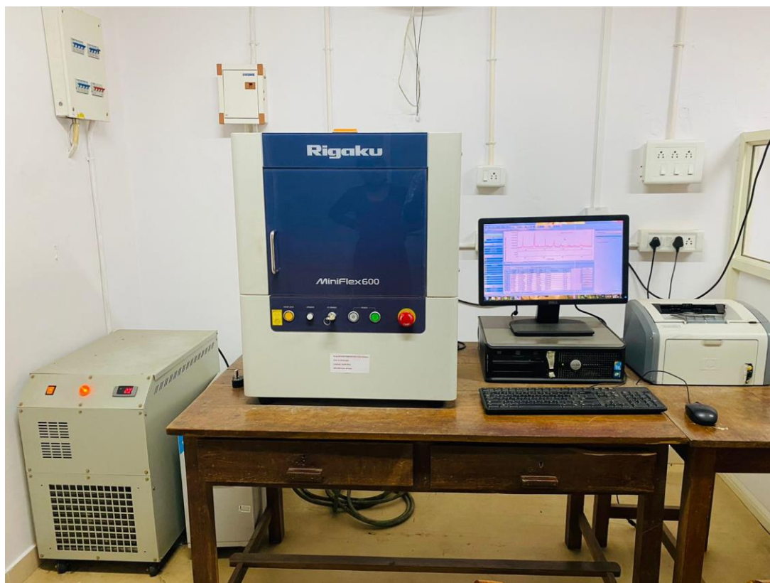
Fig 2.4 Rigaku Miniflex X-ray diffractometer
