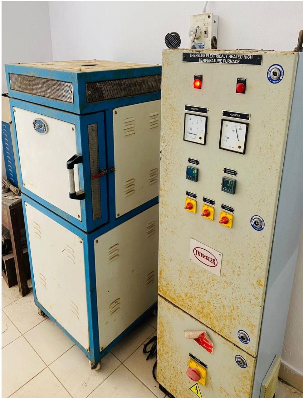
Fig 2.1 Therelek electrically heated high temperature furnace
