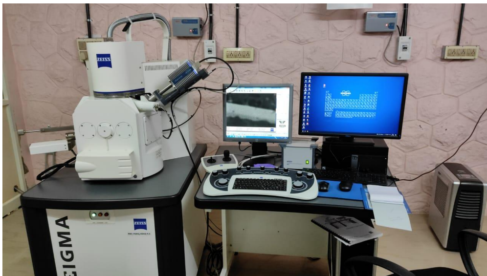
Fig 2.6 Carl Zeiss Sigma model FESEM with EDAX facility
