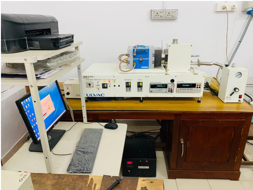
Fig 2.9 ULVAC ZEM-3 (M8) measurement system
