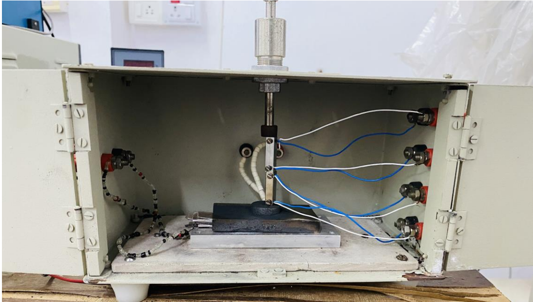
Fig 2.12 Thermal conductivity measurement set up
