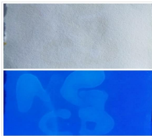
Figure 4.8: Photographs of filter paper written using MGCDs solution under day light and UV light
