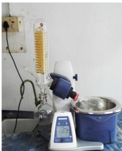
Fig. 3.1. Extraction of microbial IAA from the ethyl acetate fraction using rotary evaporator
