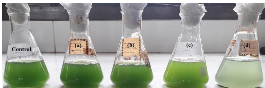
Figure 9.4: Dose-dependent study of CuNi BNPs on Algal growth, where (a), (b), (c), and (d) are displaying the effects of 0.5, 1, 2, and 3 g of BNC, respectively, on the 12 th day.
