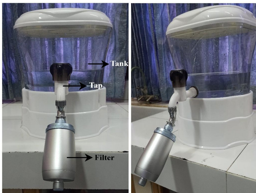
Figure 8.1: Photographs of the apparatus for the water purification device used for filtration containing lead, cadmium, manganese, and zinc contaminated water.
